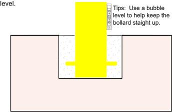
Step 6. Patch the surface around the pipe bollard to make it smooth with the ground. Wait until the cement is cured. Replace the top cap. The installation is completed.
